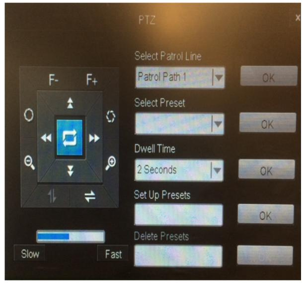
Using this controller, you can move the camera to the desired position, enter numbers between 1-16 in the "Set Up Presets" field to program "Patrol Path 1". Once you have the presets entered, click OK next to "Patrol Path 1" and the camera will begin the tour. "Patrol Path 2" uses presets 17-32.
