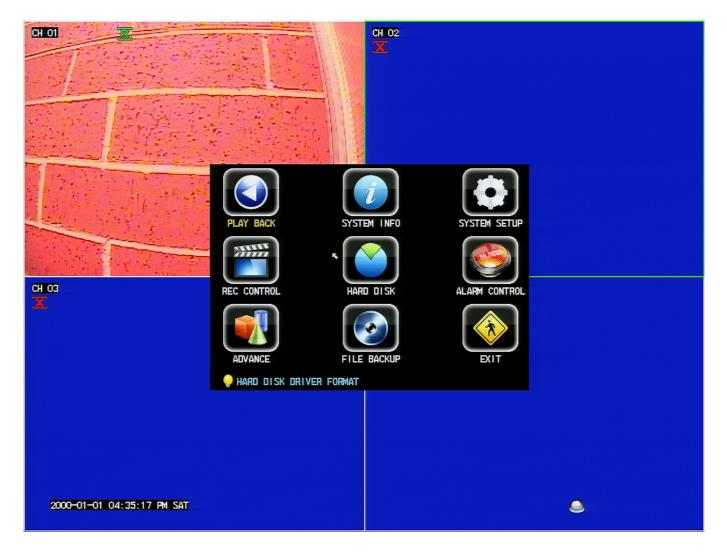
You will be given the file backup menu as shown below. Before proceeding insert your USB flash drive in the free USB port on the back of the DVR. Press the "detect" button as shown in the menu below. If your USB device is not found try swapping Page 3 / 7
