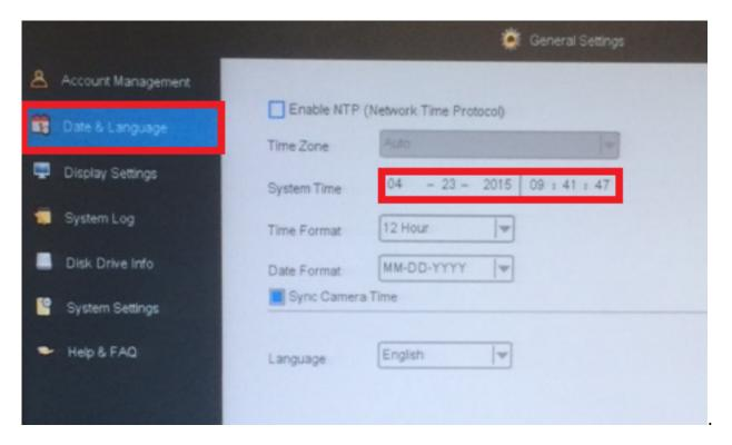
The "System Time" must be set in using a 24 hour clock.
