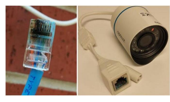
To weatherproof the cable ends, you can either tape the cable ends or install the cable ends into a conduit box. By far the safest option is to install the cable ends into a conduit box to protect the cable ends from the rain and wind.
