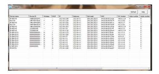
You can then open Internet Explorer to access the cameras settings using the camera's IP address.
