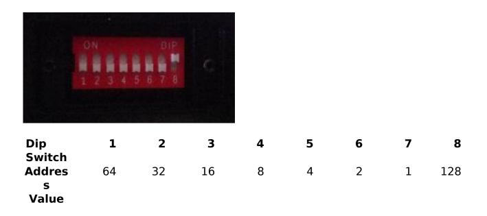
In order to confirm the addressing has been set, you must **call** preset 140 from the DVR/Joystick **after** camera has been powered off and on
