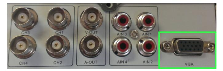
If the cable is plugged in properly, then you must try to reset the resolution to defaults.
