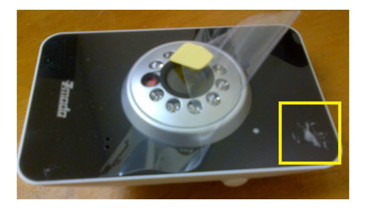
Next, use pliers or a similar metal tool to pull up the lose plastic section from the second clear plastic cover:
