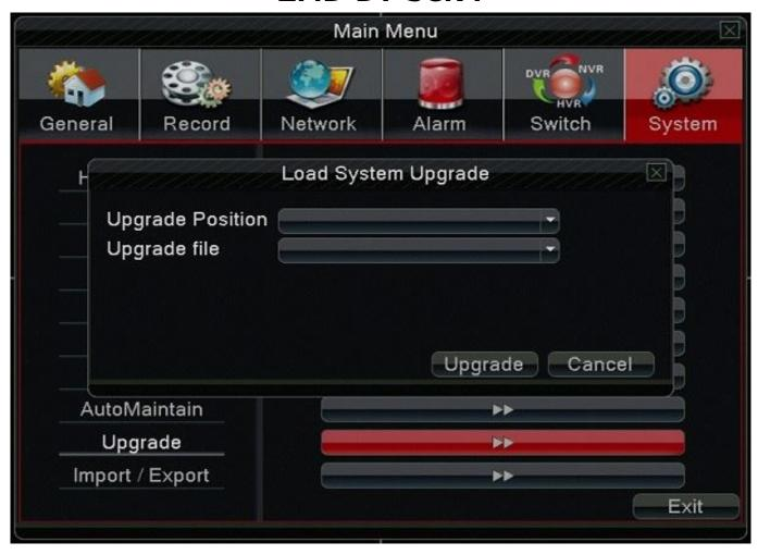
From this menu, select "Upgrade" and do not power off the DVR until the update is completely finished loading. The DVR will reboot at least one time during the update process.
